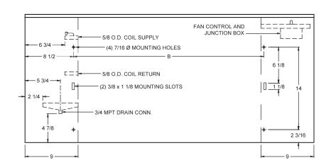
LEFT HAND PIPING CONNECTIONS SHOWN. RIGHT HAND OPPOSITE. PIPING HAND DETERMINED WHEN FACING AIR OUTLET ELECTRIC JUNCTION BOX LOCATION MAY VARY DEPENDING UPON CONTROL REQUIRMENTS. CONTACT FACTORY.
